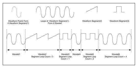
Figure 17-1. Examples of Waveform Generation
