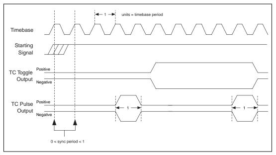
Figure 7-2. Am9513 Counter Timing and Output Types
