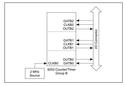
Figure 2-2. Lab and 1200 Devices Counter/Timer Signal Connections
