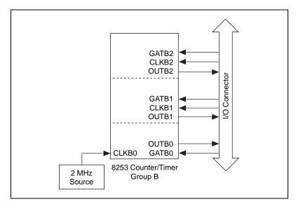
Figure 3-1. LPM Device Counter/Timer Signal Connections
