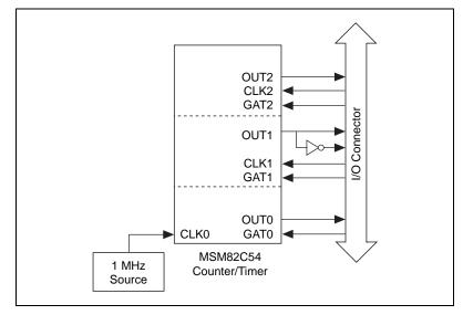
Figure 4-1. DAQCard-700 Counter/Timer Signal Connections
